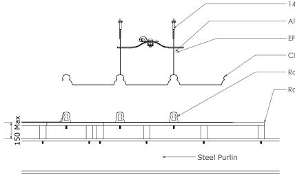
14G x 75mm Tek Screws into Roof-spacer
