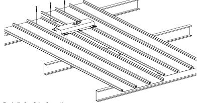
Details for <u>3 to 9 purlins</u> Min 3 Fixings into purlins - Fixings into purlin above or below anchor plate (closest purlin to anchor plate). MIN 12 Rivets required in Anchor Plate <u>10+ Purlins</u> - No additional fixings required
