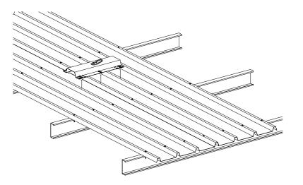
Minimum 3 Purlins Anchor riveted through lap (fixed over 2 roof sheets) QTY 12 x 8mm Bulb type Rivets required in Anchor Plate
